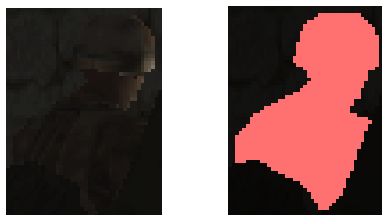
Figure 10: Contrast-enhanced normal-color image at left showing a highlight on the helmet that raises the average brightness of the target enough to confuse the algorithm. Corresponding false-color image at right.
